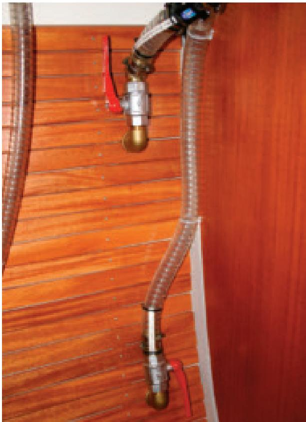
*Easy access to well dimensioned ball valves for through-hull fittings*
