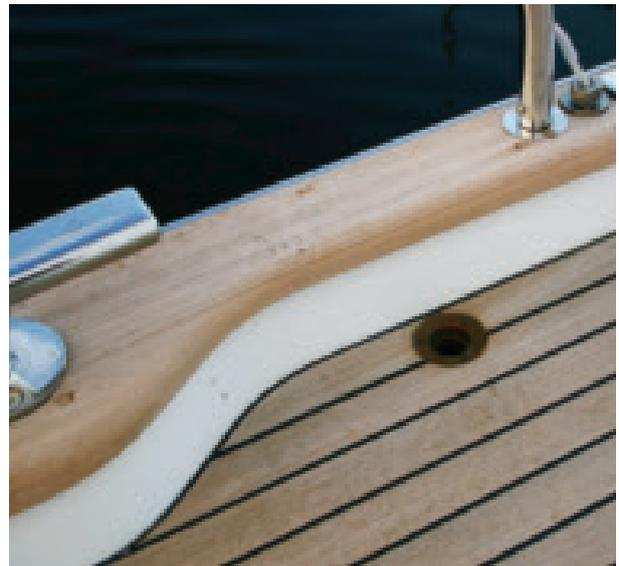
*Deck drains with exits under the waterline, to prevent dirt strips on the hullside (HR 342 and larger)*
