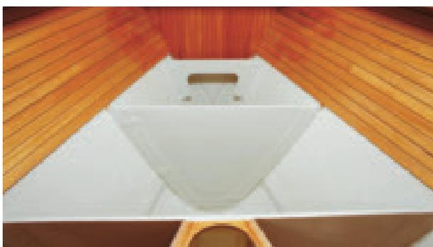
*The forward section is stiffened by additional bulkheads below the berths*
