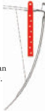
The chain plates are secured to the insulated hull through guides that are inclined so that there is no change of angle throughout their length.
