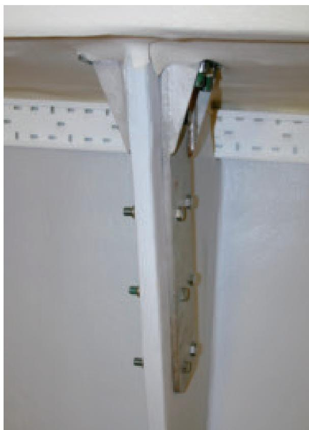
*The support for the rigid stainless chainplates is laminated from both sides to the hull and to the deck to distribute loads*
