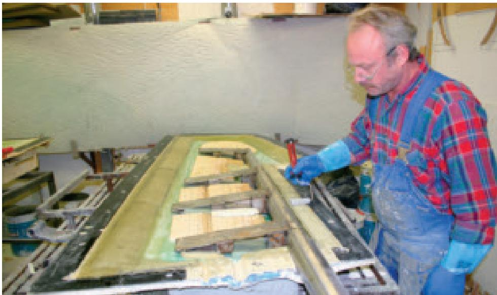
*The rigid rudder has a solid stainless shaft (no pipe) that is casted into the solid rudder blade*
