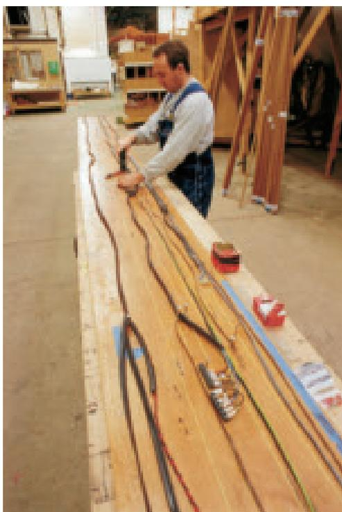
*Wiring is prepared outside the boat*
