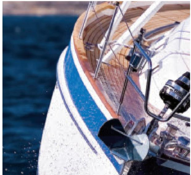
*A sturdy rubbing strake is integrated to the hull*
