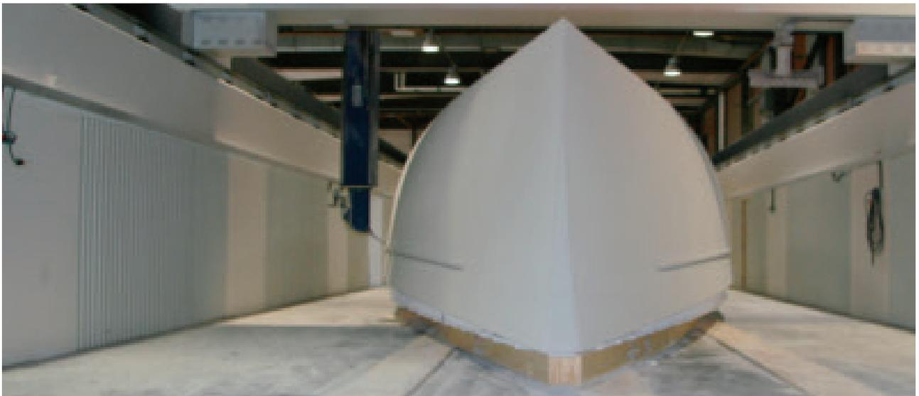
*The plug takes shape in a CNC milling machine*
