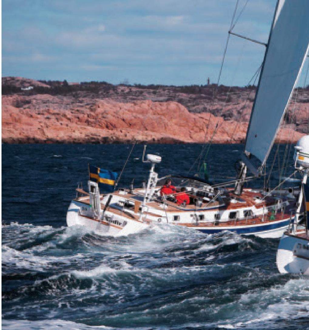
*Above: three HR 62s with sails hydraulically furling and reefing from push-buttons at the steering stand; the winches are also powered. A mere fingertip movement control even the biggest yacht*
