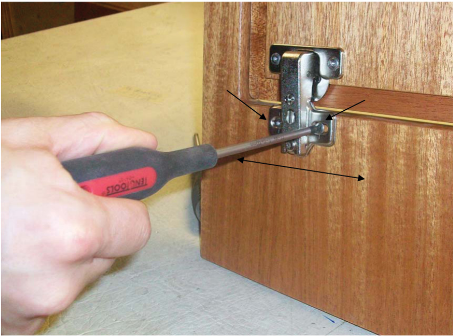
To adjust the hinge from side to side, use these two screws
