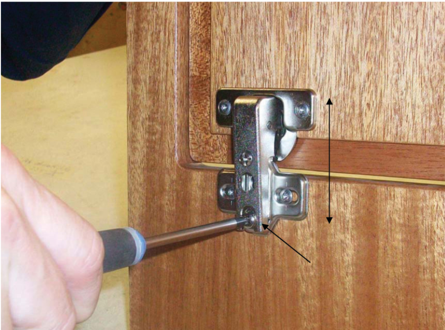
To adjust the hinge up and down, use this screw
