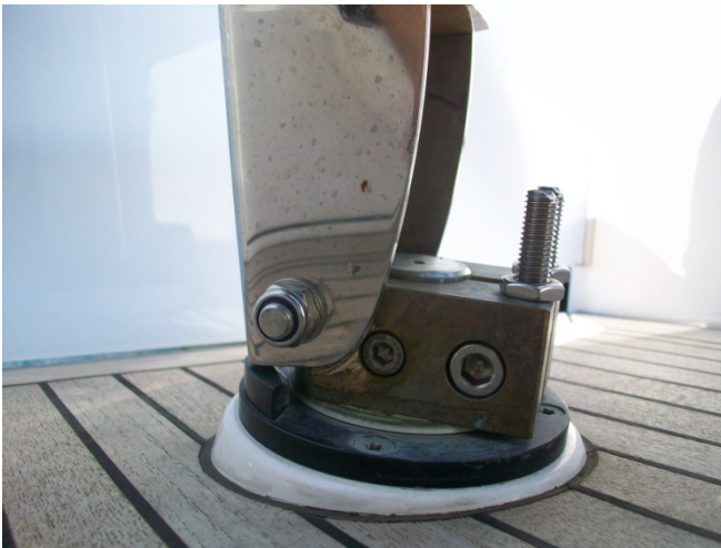
Hallberg-Rassy 310 upper rudder shaft fitting
